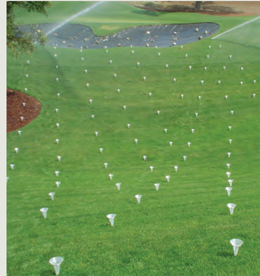
An irrigation efficiency test at a local golf course.
