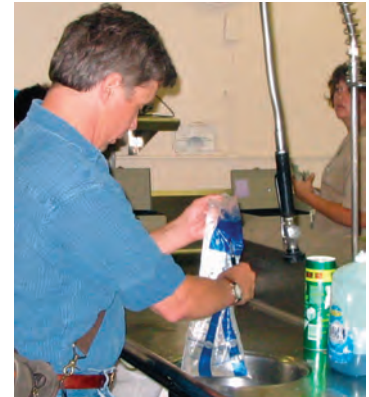
Surveyor checks efficiency of a pre-rinse spray valve at a local high school cafeteria.
