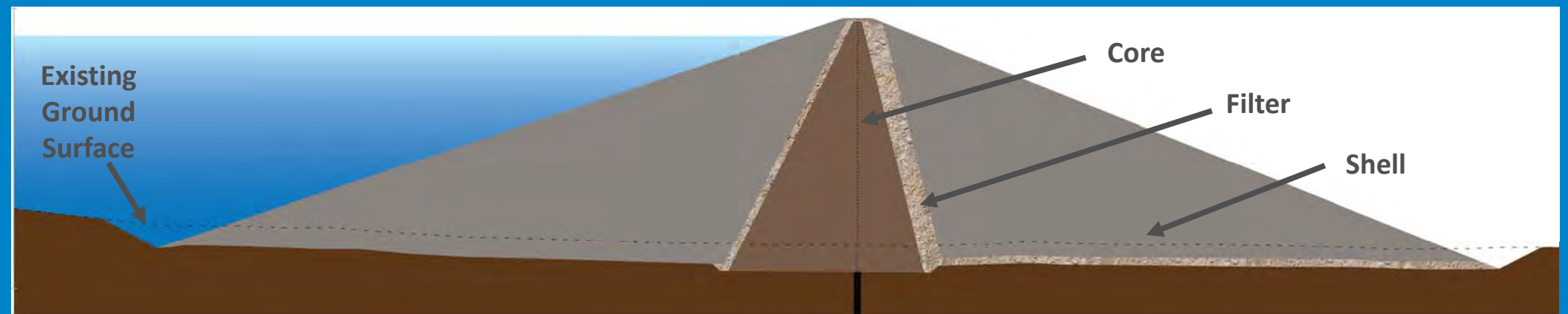
Typical Earthfill Dam Cross Section
